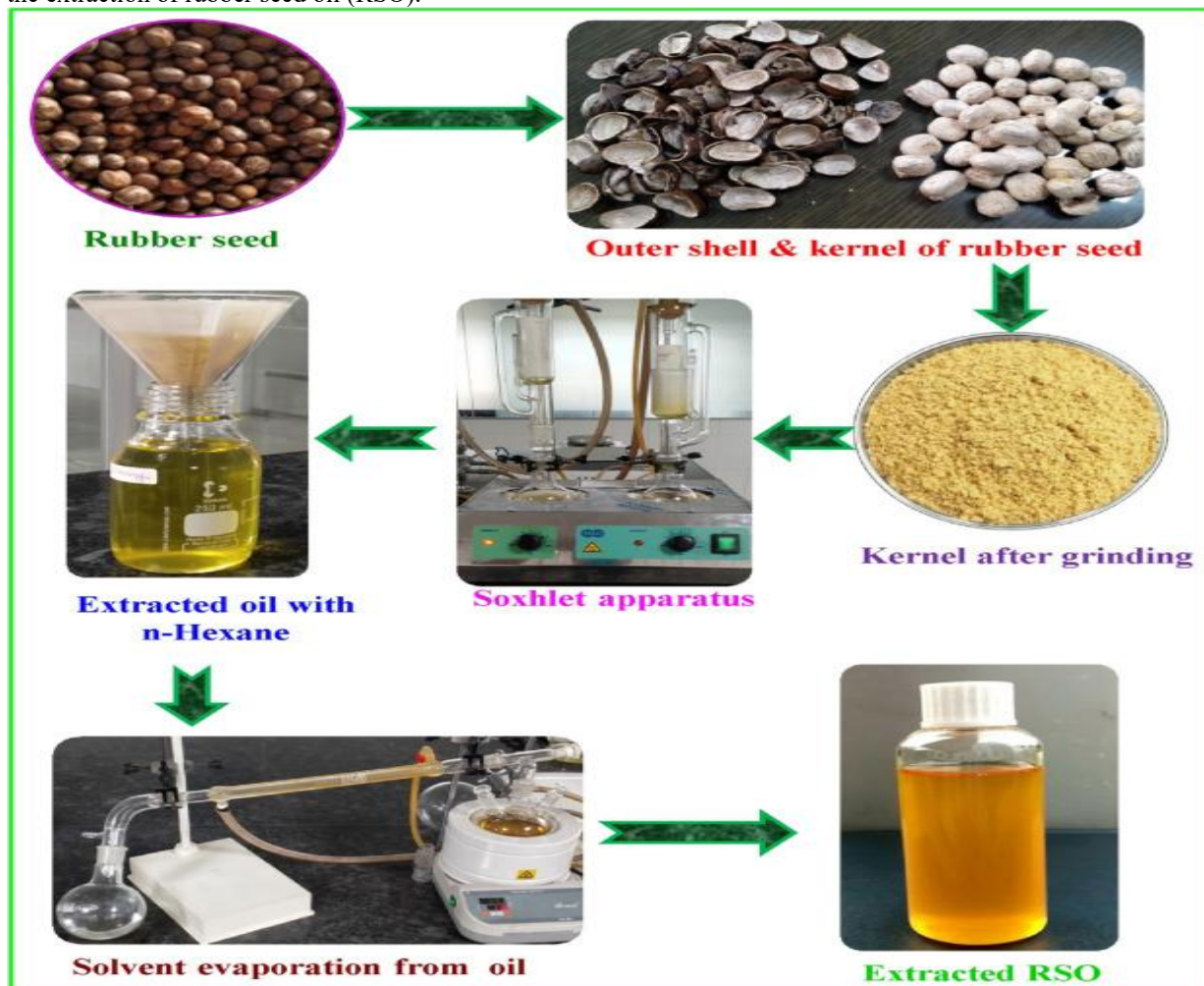
Figure 3. Schematic representation of the extraction of RSO [16]
